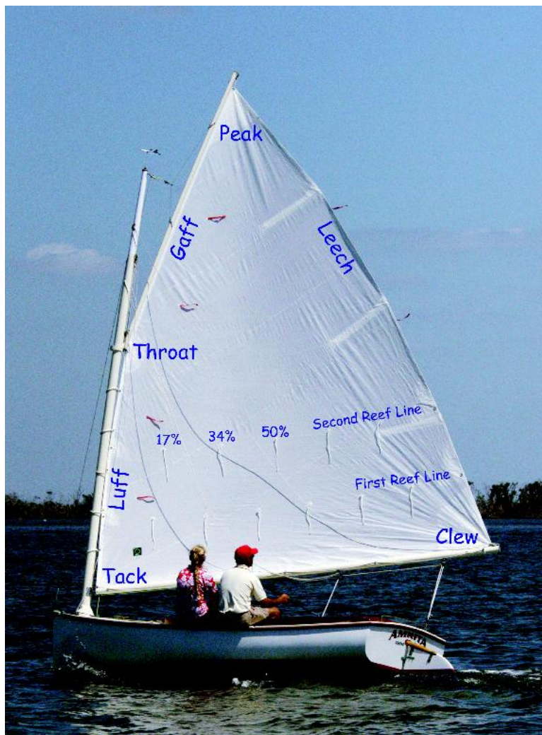
A look at the parts of a four-sided gaff-rig sail reveal similarities to the more familiar three-sided sail, with a few additional points. The reef points divide the sail lengthwise, and can be used to measure the position of the draft.
