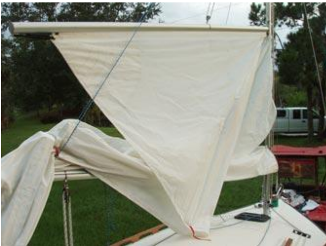
Sail partially raised showing lazy jacks holding main boom and constraining gaff boom and part of sail
