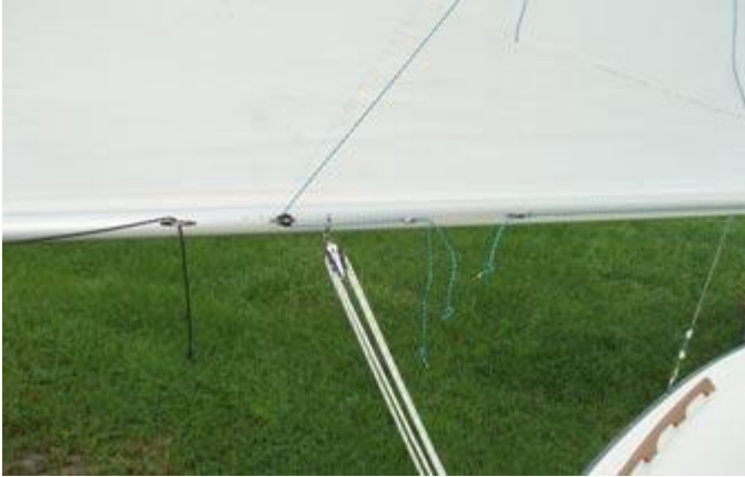
Cleat for clew reef, block for lazy jack, cleats for lazy jack and reef line
